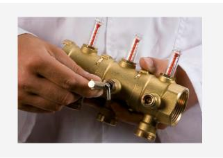
Known the flow rate that must pass through the circuits connected to the manifold, with circulator operating and any interceptions on the return manifold kept open, remove the protection cap on the front of the modules and then use the R558 key to completely loosen the mechanical memories and lockshields.
