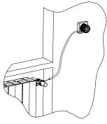
**6)** Install the adjustment knob at the desired distance, using the installation kit included with the package.
