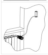
**5)** Install the sensor on a wall, at a height of around 1,5 m from the ground, using the installation kit included with the package.
