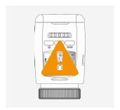
▲ This position is not recommended due to the influence of the radiator temperature on the chronothermostat.
