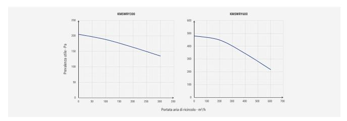
Loss of pressure on air circuit based on total air flow rate.
