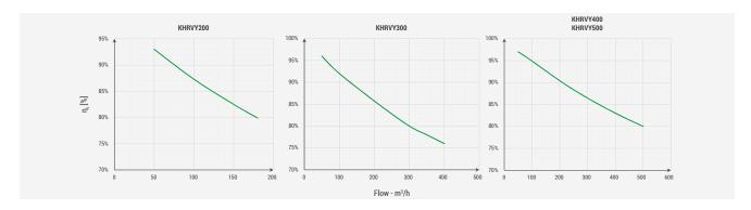
Efficiency curves, version with standard exchanger.
