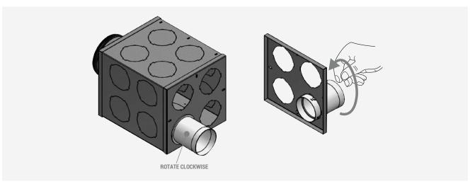
Installation of initial adapter in plenum/manifold hole.
