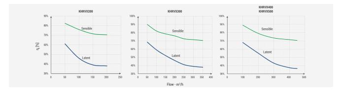
Efficiency curves, version with enthalpy exchanger.
