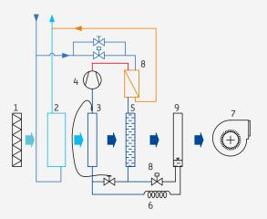
Fig. 2: schematization of a sensible integration dehumidifier.
