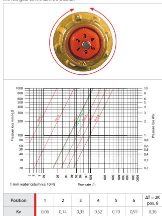
The condition  $\Delta T$ =2 K pos.6 refers to the hydraulic conditions when a Giacomini thermostatic head is installed and the pre-regulation is set to the position No. 6 (maximum opening degree).
