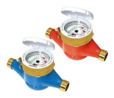
Domestic water meters for boiler room, GE552-3 series, with male threaded connections, multi jet, dry dial and direct reading on five/six numberic rolls, equipped for M-Bus data centralization through M-Bus module. Available in versions for domestic cold water (50 °C) and domestic hot water (90 °C).
