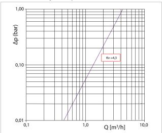
Figure 16 – Check valve, code R189VY004
