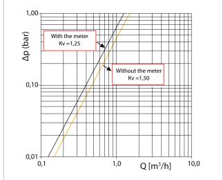
Figure 11 – Sanitary hot water (SHW)
