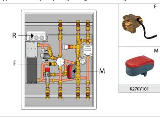
Figure 17 – Positioning of optional accessories for priority sanitary water management
