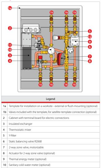
Differential pressure control valve, R147N Figure 2 - GE556Y303 satellite with optional accessories
