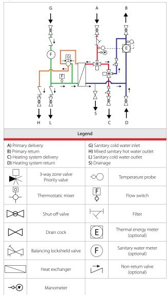
Figure 3 – Operation diagram
