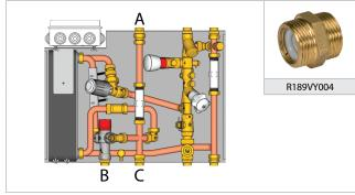
Figure 18 – Positioning the sanitary water check valves (optional)
