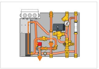
Figure 13 – Sanitary hot water (SHW)
