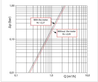
Figure 7 – Sanitary hot water function – primary side
