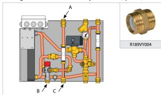
Figure 15 – Positioning the sanitary water check valves (optional)
