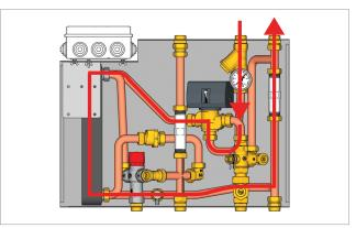
Figure 7 – Sanitary hot water function – primary side
