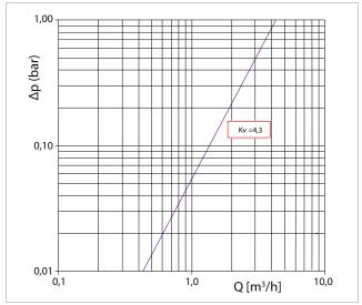
Figure 14 – Check valve, code R189VY004
