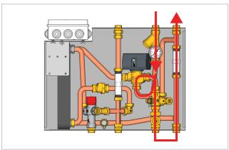
Figure 5 – Heating function – primary side
