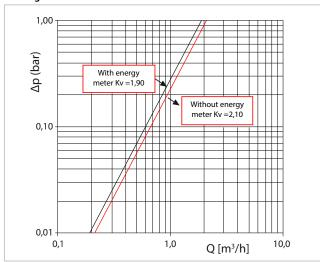
Figure 4 – Heating function – primary side
