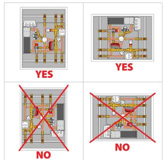
Figure 14 – Correct and incorrect assembly
