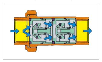
In the case of depression upstream or increase in pressure downstream, the check valves are immediately closed, preventing downflow.
