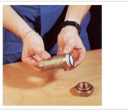
3) check that the two check valve modules are in perfect working order; there should be no impurities on the seal housing or on the closure spring. If the modules are worn, replace them.
