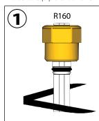
Before screwing the R160 valve, verify that the plastic paddle does not interfere with the parts inside the seat, it is necessary to have a free space of at least 35 mm. If any interference is present, cut the exceeding part of the paddle with a shear.
