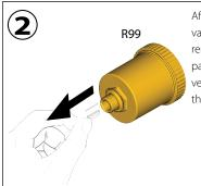
After the screwing of the R160 valve on the installation seat, remove the possible plastic paddle of the automatic air vent valve and proceed with the assembly.
