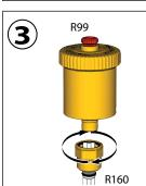
Screw the automatic air vent valve to the R160 valve, by making the plastic paddle be guided by the hole of the body of the automatic air vent valve.
