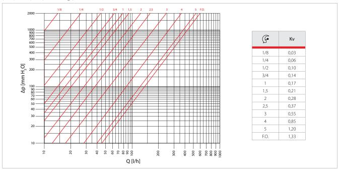
Balancing on the lockshield of the delivery manifold in the thermostat-controlled version with R463 thermostat-controlled actuators assembled, in opening conditions corresponding to  $\Delta T = 2$  K.
